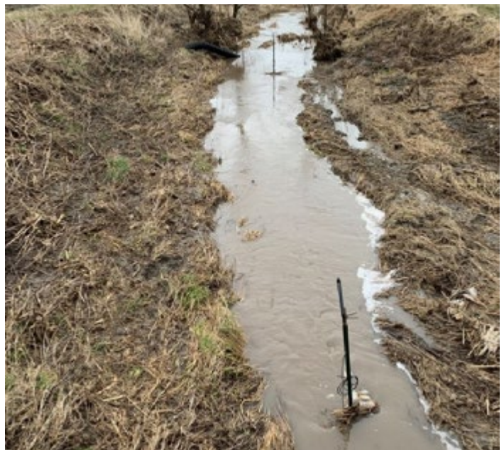
Figure 5. Pair of Onset pressure transducers used to monitor surface water level and flow.
